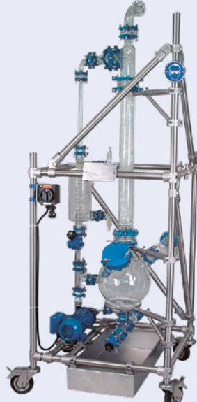
Mobile gas scrubber Mobiler Gaswäscher
